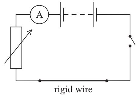
With the switch open, the balance was set to zero. When the switch was closed a current  $I$  in the circuit was recorded by the ammeter and the reading on the balance increased.
