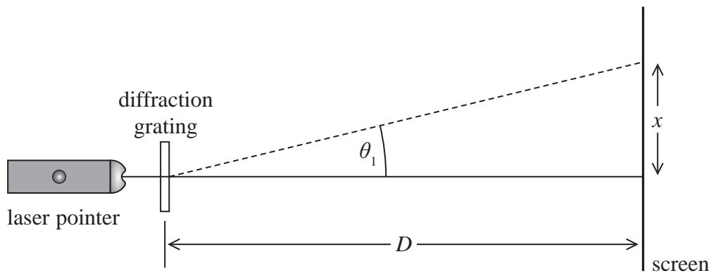
The distance between the first order maximum and the central maximum of the diffraction pattern was  $x$ . The distance between the diffraction grating and the screen was  $D$ .
